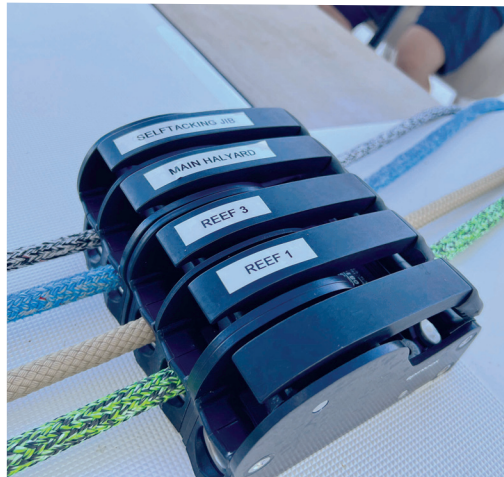
◀ All halyards return to the helm stations and all lines are easily accessible.
