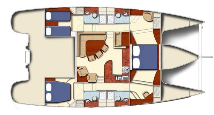
The Master cabin is forward and there are two double cabins aft. One in each hull.
